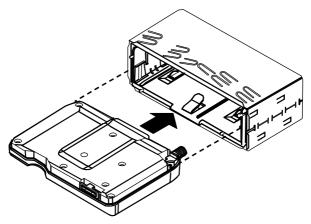
7. Place the front panel onto the bracket. Push firmly until the four locking studs click into place.
